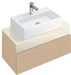
MEMENTO VANITY C780 U0 FC (W) 31 ¾" x (H) 14 ¾" x (L) 18 ¼" 1 drawer with soft-closing system 1 pull-out compartment For combination with Memento washbasins 5133 U8/UA/UC 23 ¾" x 16 ½"
